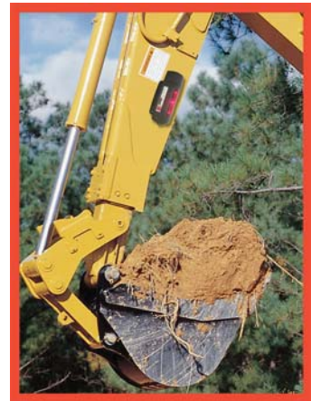
MP1 mounted to a backhoe boom
