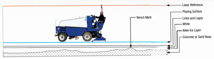
Level-lce literally takes all the guess work out of producing a perfectly level sheet of ice. The laser controlled ice leveling system provides accurate reference point to within .5 mm. Using the most advanced receiver technology, the system controls the cutting blade of the conditioner to give your ice a perfectly level surface after every flood.
